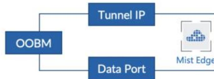
**Data Port** is connected to a trunk port that has all the VLANs configured where the WLAN need to be mapped to
